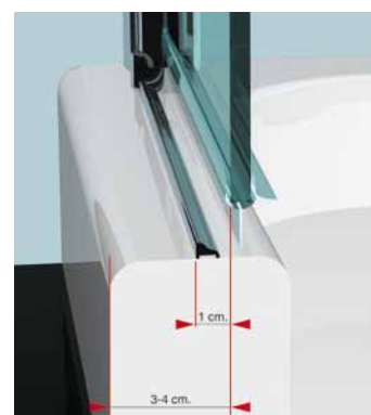
Water brake dimensions and installation
